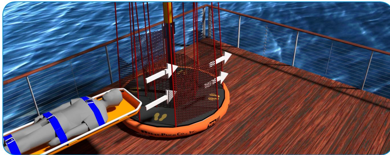
2. Vertical grab lines will expand to accommodate the width of the stretcher.
