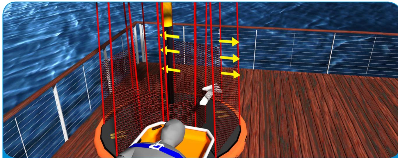
Vertical grab lines expand when stretcher is carried through opening
