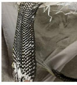
Figure 2: Failed Lifting Point
