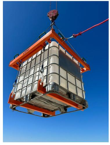
**IBC Lifting with Pallet Bars**
